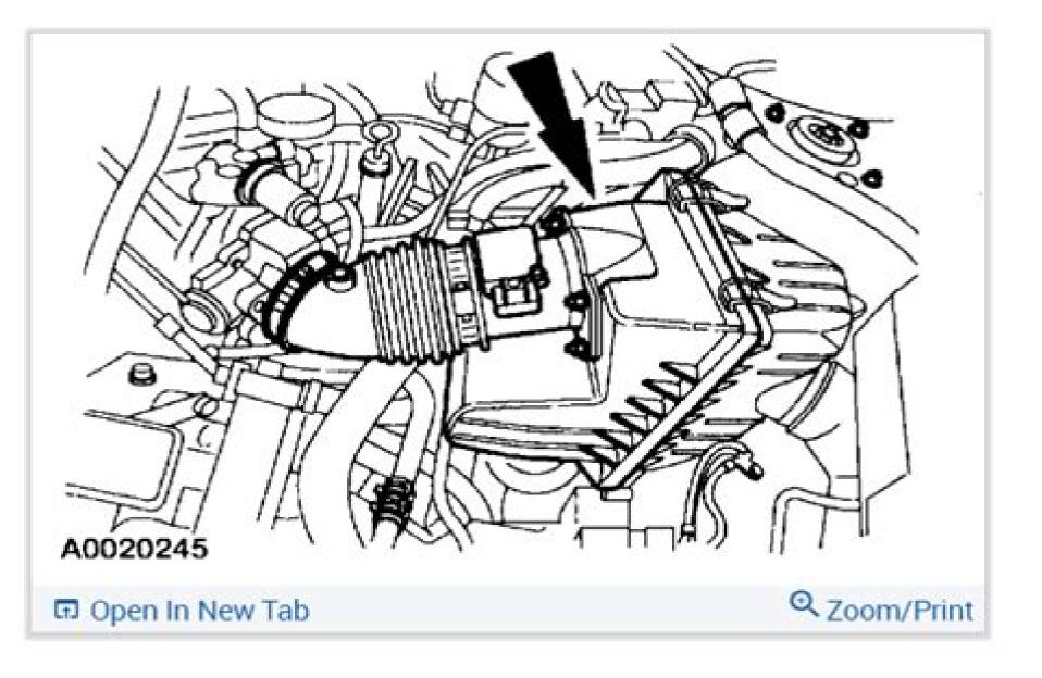
4. Remove the intake tube and air cleaner cover.
