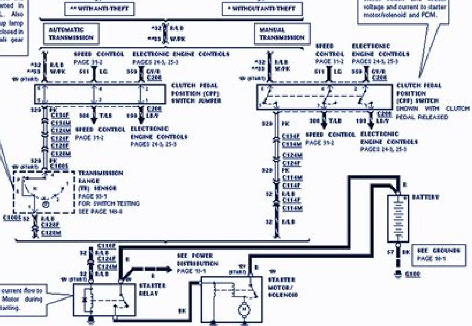
Controls current flow to Starter Motor during engine starting.
