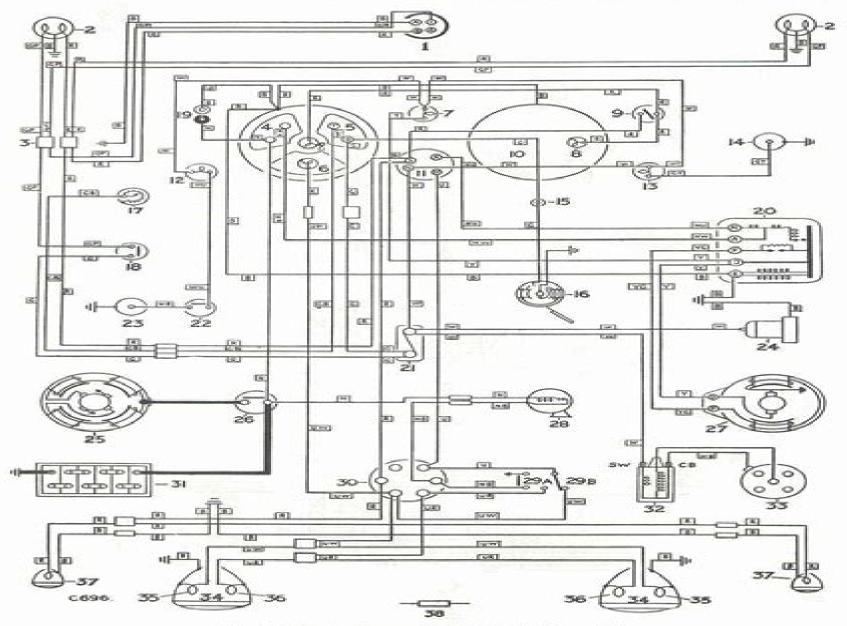
Fig. P-8—Wiring diagram 88 and 109—1954-58 models See Page P-9 for key to wiring diagram
