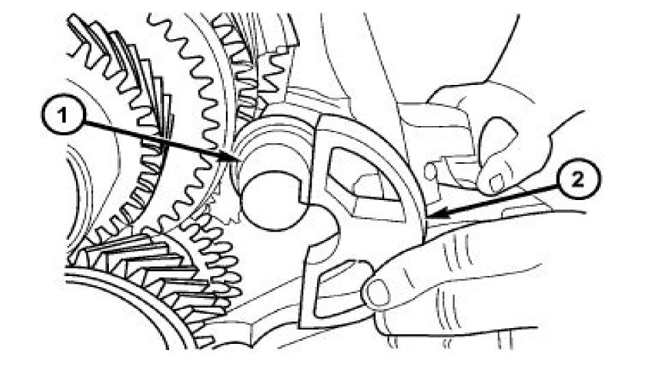
Fig. 25 IDLER SHAFT SUPPORT
