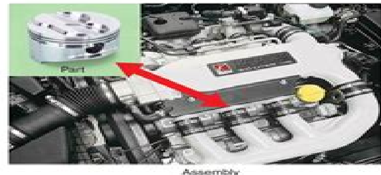
Figure 1-1. An assembly is a group of parts that work together to perform a function. For example, an engine is an assembly that contains pistons, which convert the fuel's heat energy into useable kinetic energy (motion). As you will learn, an engine has many other parts. (Saturn)
