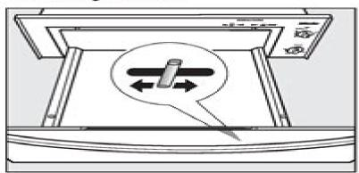
The humidity control adjusts the humidity within the drawer. The humidity control can be set anywhere between "Moist" and "Dry".
