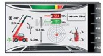
Continuously analyzes the position of your load in accordance with the machine's work configuration. The system restricts the working area based on the accessory used and load being handled.
