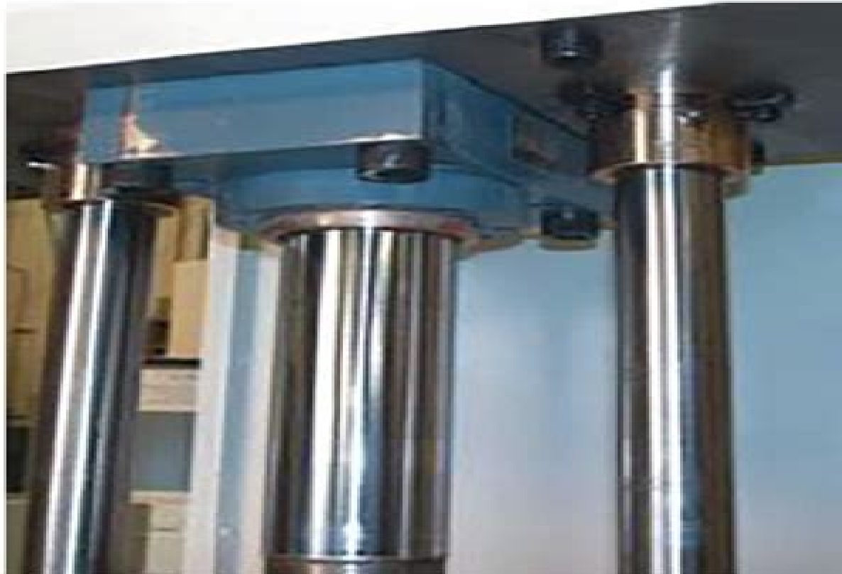
Figure 1: Replace the ram seal when drops of oil are visible on the ram itself. The ram should run dry or with a very light, even film of oil on it. Bronze bushings should be greased as necessary.
