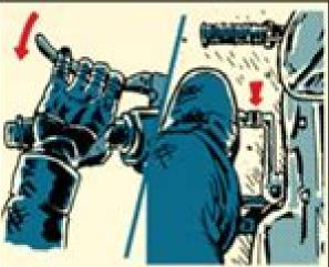
Squeeze in the clutch lever and press down on the gear shift lever to reach 1st gear.
