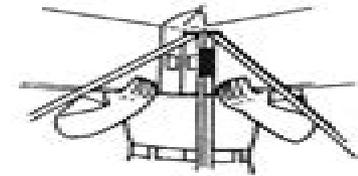
3. Attach Velcro on each corner and then pull the frame completely open.
