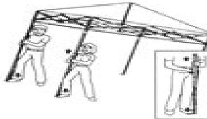
5. Lift each leg until the buttons snap into the first hole.
