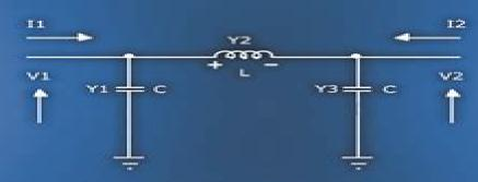
$$\begin{bmatrix} Y \end{bmatrix} = \begin{bmatrix} Y_{11} & Y_{12} \\ Y_{21} & Y_{22} \end{bmatrix} = \begin{bmatrix} Y_1 + Y_2 & -Y_2 \\ -Y_2 & Y_2 + Y_3 \end{bmatrix}$$
