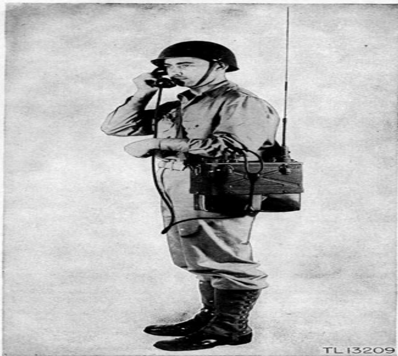
Figure 19. Radio Set SCR-300-A, lightweight installation.
