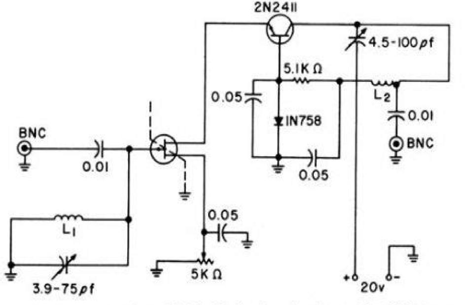
L<sub>1</sub>, L<sub>2</sub> 18 turns B&W 3004 Minductor; L<sub>2</sub> tapped 13/4 turns from ground.
