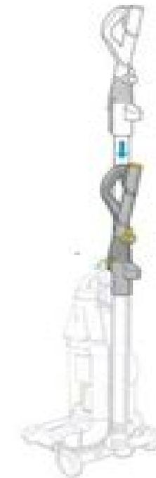
Slide wand into top of machine and click into place.
