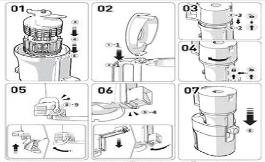
01 Place the bottom part of the multi-screw (3) into the chamber (3), insert the top part of the multi-screw (3) as shown in the image, and then firmly press the assembled multiscrew set.
