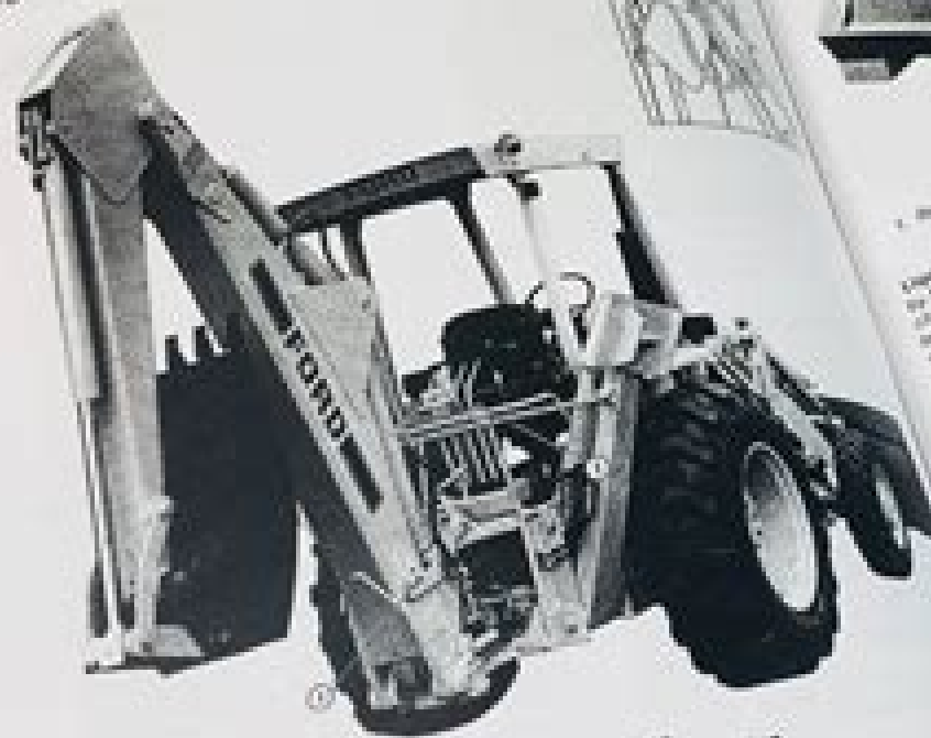
Figure 26 Backhoe in Transport Position 1. Boom and Swing Transport Lock 2. Stabilizer Transport Chain 3. Extendible Dipstick Pinned and Lock
