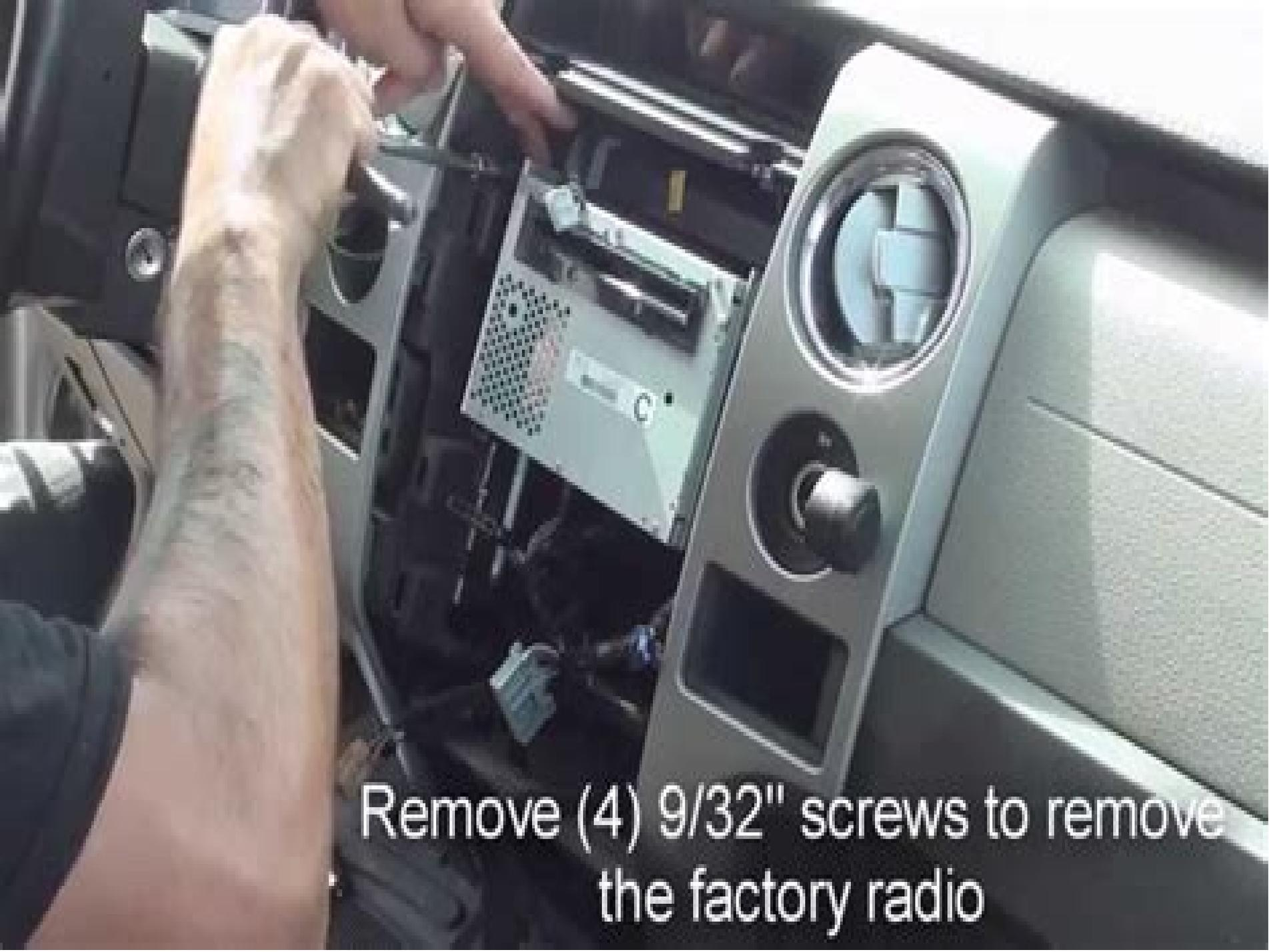
Remove (4) 9/32" screws to remove the factory radio
