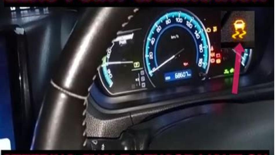
STEERING ANGLE SENSOR LIGHT ON
