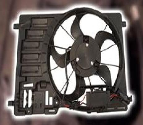
HOW TO REPLACE ENGINE COOLING FAN ASSEMBLY 2013-2019 FORD ESCAPE 2.0L L4
