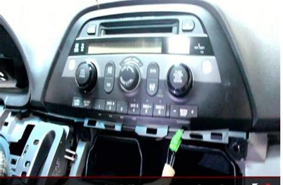
Remove screws holding stereo in place. Screws have been removed in the video
