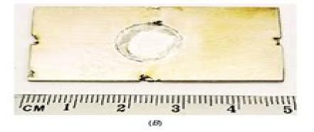
critical crevice temperature (CCT) of a material. In the standard, the CCT is defined as the minimum temperature, in degrees Celsius, to produce crevice attack at least 0.025-mm deep on the bold surface of a specimen beneath the crevice former, ignoring edge attack. The methods also can be used to rank alloy performance, aid in materials selection, and the design of new materials. 10,100-11
