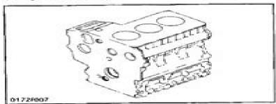
The engine has a highly durable tunnel-type cylinder block in which the bearings, pistons, crankshaft and camshaft are installed.
