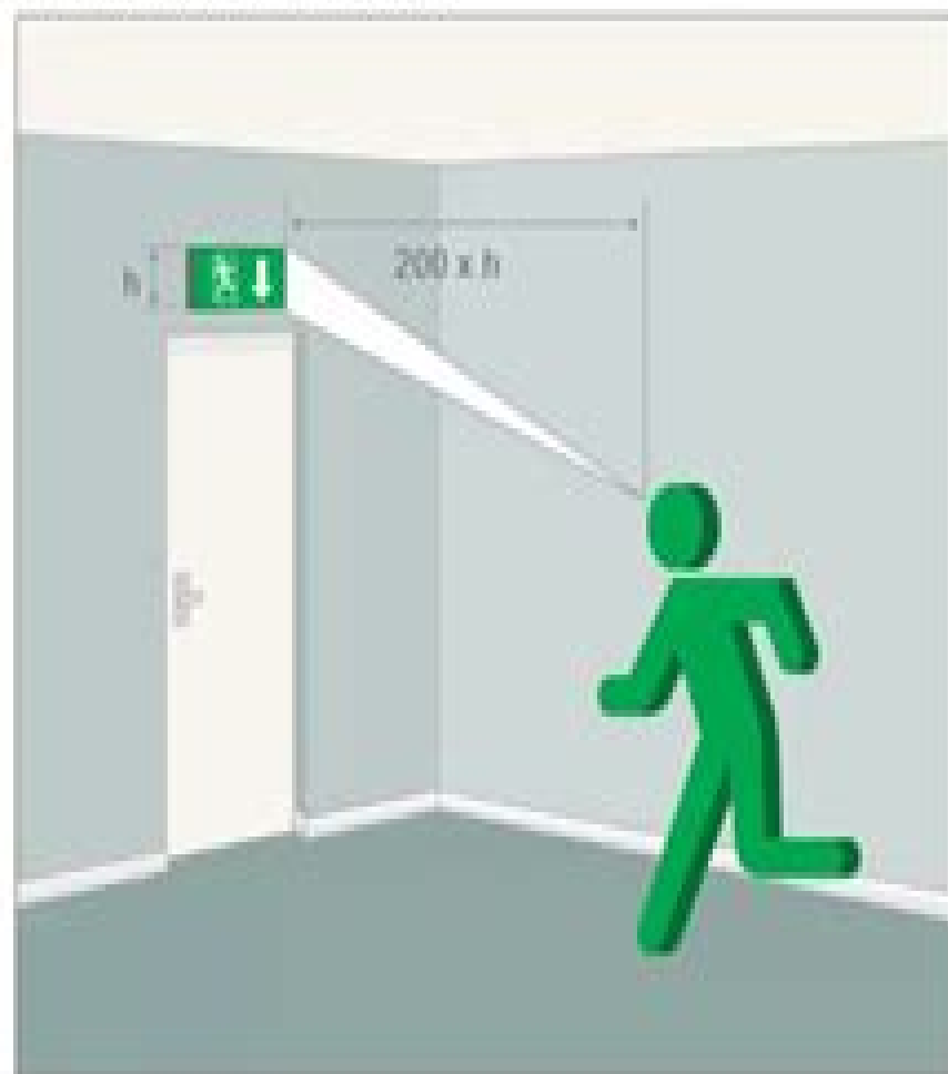
Internally illuminated signs - 200 \times the panel height
