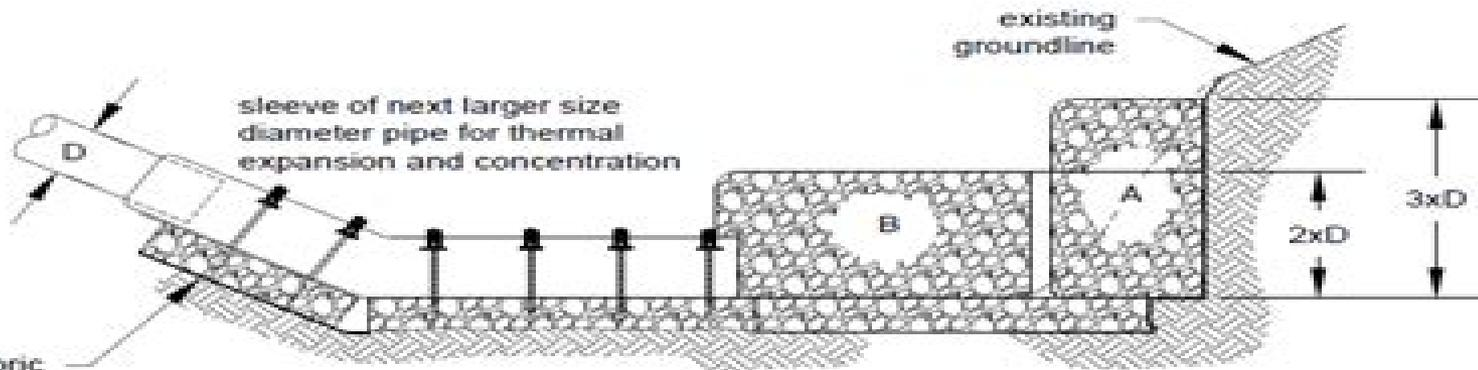
place filter fabric between gabions at soil bedding
