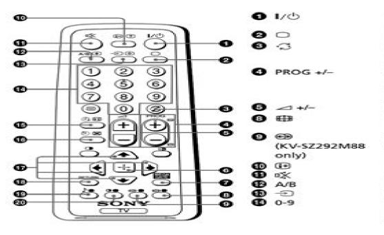
Turn off temporarily or turn on the TV. Display the TV program. Jump to last program number that has been watched for at least five seconds. Select program number. To select quickly, press and hold until the desired program number appears. Adjust volume. Change the picture size: "On" (16:9 wide mode), "Off". Select surround mode options (see page 13).
