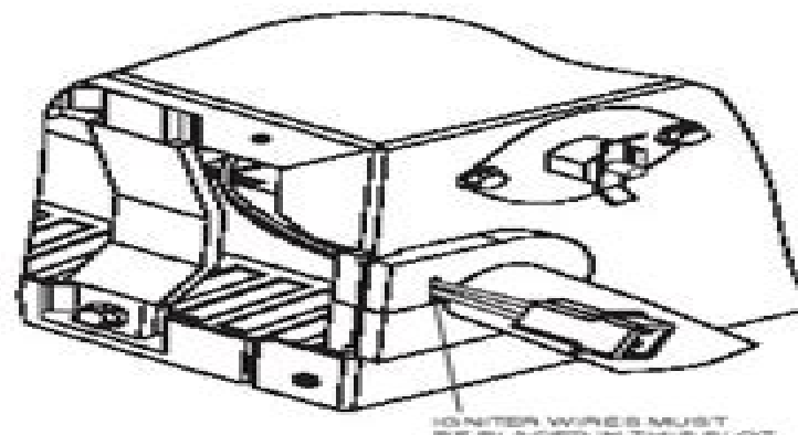
Fig. 7 - Igniter Wire Placement
