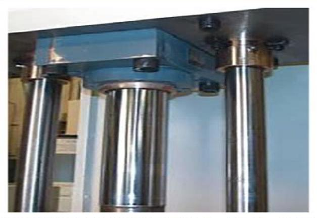
Figure 1: Replace the ram seal when drops of oil are visible on the ram itself. The ram should run dry or with a very light, even film of oil on it. Bronze bushings should be greased as necessary.
