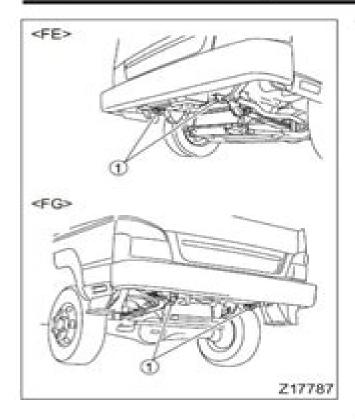
Never use the tie-down hook(s) ① under the frame for towing purpose. The tie-down hook is to secure the vehicle when transporting it. If the hook is used for towing, damage to the front bumper or frame may result.
