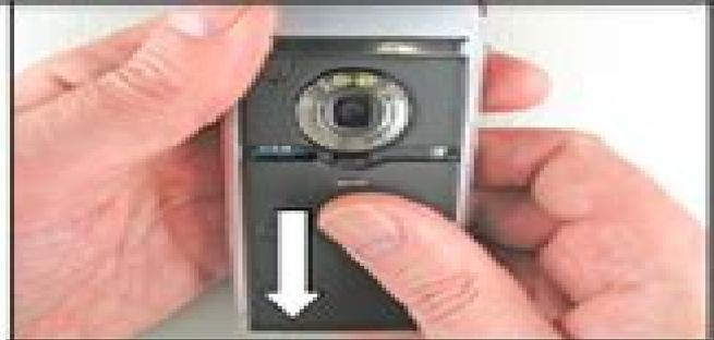
Remove the battery lid completely.
