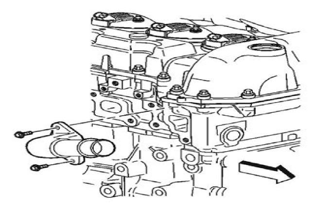
Fig. 41: View Of Water Outlet Courtesy of GENERAL MOTORS CORP.
