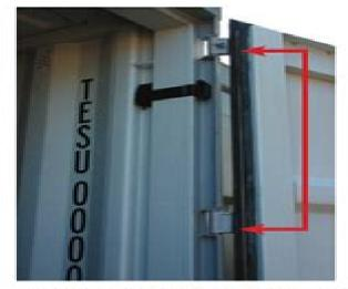
Place the CSD between these two possible locations, between the top and second hinge but not directly touching the hinges.
