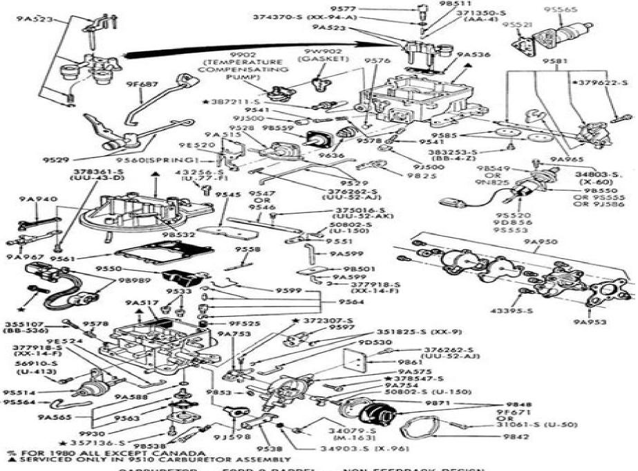
CARBURETOR — FORD 2 BARREL — NON FEEDBACK DESIGN 1980/86 6 CYL. 171 (2.8L), 230 (3.8L), 8 CYL. 255 (4.2L), 302 (5.0L), 351M (5.8L), 351W (5.8L) and 400 (6.6L)
