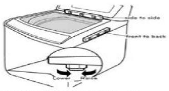
If the washer is not level, adjust the leveling feet. Turn clockwise to raise, counterclockwise to lower.
