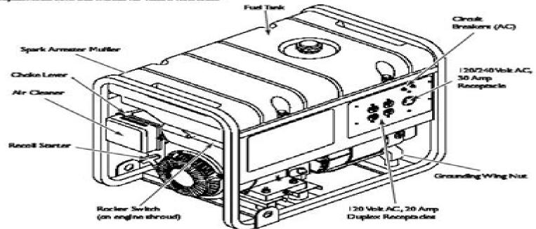
120 Volt AC, 20 Armp, Dupliex Receptacies — May be used to supply electrical power for the operation of 120 Volt AC, 20 Armp, single phase, 60 Hz electrical lighting appliance, tool and motor loads.
