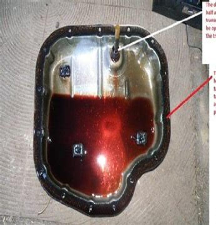
The drain tube does not allow for more than half a litre of oil to be drained out of the transmission, therefore the chamber needs to be opened up in order to completely drain the transmission.
