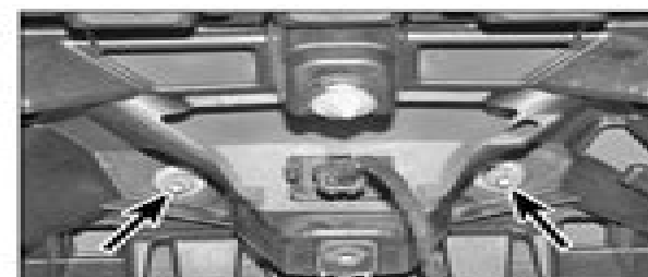
16.17 Tailgate switch/handle retaining nuts (arrowed)
