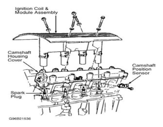
Fig. 12: Camshaft Housing & Ignition Coil/Module Assembly Courtesy of GENERAL MOTORS CORP.
