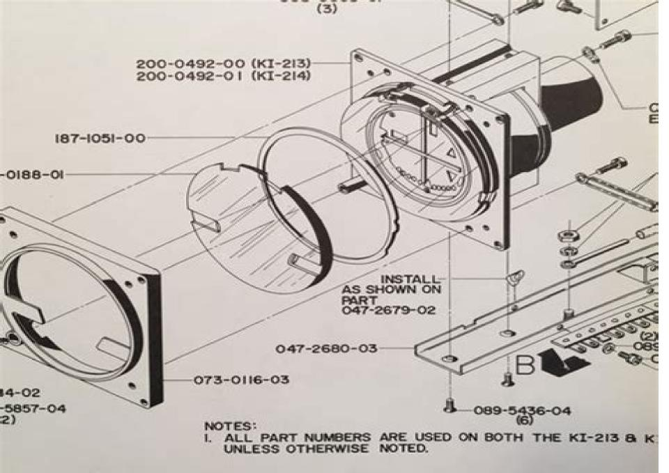
FIGURE 5-1 KI 213/214 FINAL ASSEMBLY (Dwg, No. 300-0723-00)
