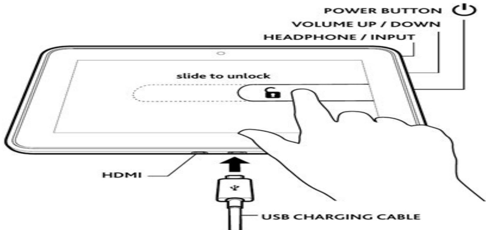
To charge your Kindle, connect it to the USB charging cable as shown. Connect the opposite end of the USB charging cable to a Kindle Power-Fast accelerated charging accessory (sold separately), or other USB power adapter. To learn more about charging accessories, visit [www.kindle.com/support/charging](http://www.kindle.com/support/charging).
