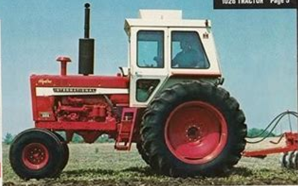
1026 HYDROSTATIC TURBO DIESEL 112.45 pto and 84.34 drawbar hp.
