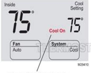
Message flashes until safe restart time has elapsed. This feature helps prevent damage to the compressor in your air conditioning or heat pump system.
