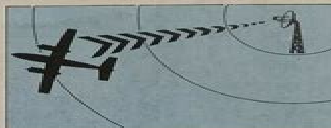
Transponder-pulsed transmitter replies to radar station.
