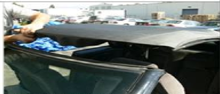
Step 28: TRIM EXCESS After dry time attach together equally and trim off excess material.
