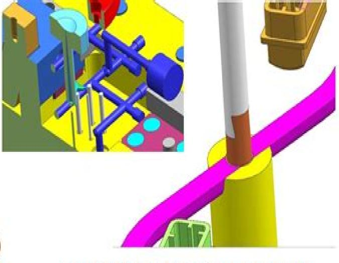
TYPES OF SPRUE PULLER IN INJECTION MOULDING
