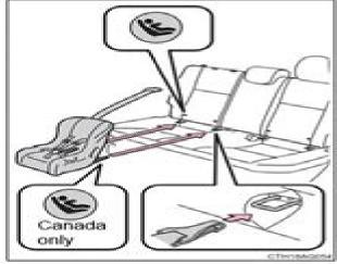
Above: This excerpt from the Owner's Manual shows the location of the lower anchors but does not mention the slit provided for easy access.
