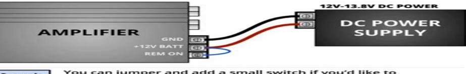
You can jumper and add a small switch if you'd like to manually turn the amp on & off. The amp won't draw any power when it's turned off even if the power supply is on.
