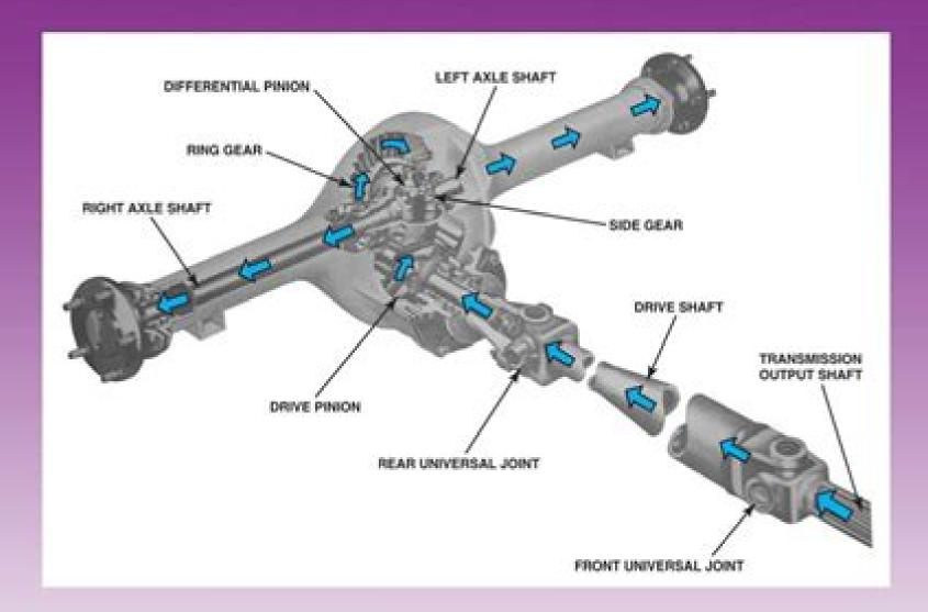
RWD drive axles have the final drive gears that turn the power flow, the differential, and two axle shafts that transfer power to the wheels.
