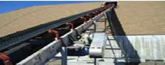
Goodyear Rubber Products stocks and fabricates heavy duty black rubber Conveyor Belting along with lighter duty constructions in both rubber and thermoplastic styles. We stock belt in large factory produced, wide rolls (slabs), slitting to our customers' required widths along with cutting to exact lengths, installing fasteners, cleats, sidewalls and/or vulcanization.
