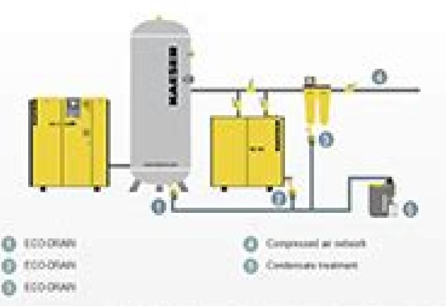
All collection points must be fitted with a reliable means of draining conductate. Best results are actioned with an electronically controlled conductable drain.
