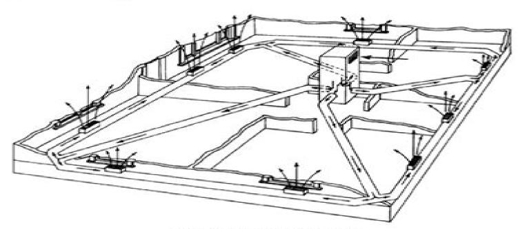
Figure 6-4. Perimeter loop delivery system.
