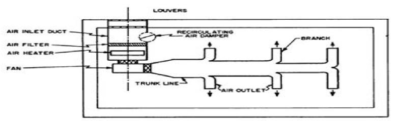
Figure 6-3. Central fan heating system.
